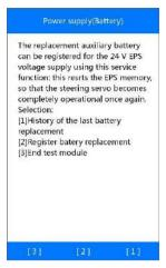
Figure 5-65 Sample Auxiliary Battery Functions
