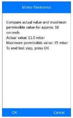
Figure 5-41 Sample Exhaust Backpressure at Idle
