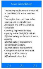
Figure 5-57 Sample Battery Replacement Registration
