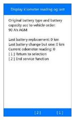
Figure 5-56 Sample Battery Capacity Screen
