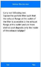
Figure 5-37 Sample Test Screen
