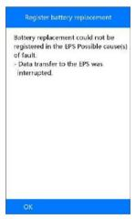
Figure 5-71 Sample Registration Failed Screen
