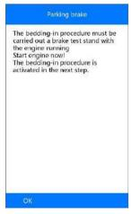
Figure 5-9 Sample Bedding-in Procedure
