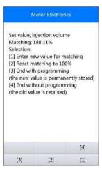
Figure 5-23 Sample Injection Rate Screen
