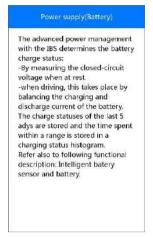
Figure 5-49 Sample Evaluate State of Battery Charge Notes
