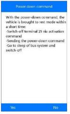
Figure 5-61 Sample Power Down Command Confirmation Screen
