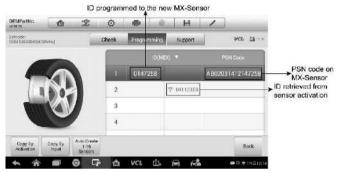
Figure 4-34 Sample Programming Screen via OEM Part No.
