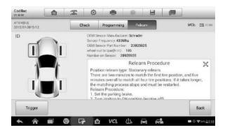
Figure 4-24 Sample Stationary Relearn Screen 1
