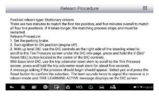
Figure 4-25 Sample Stationary Relearn Screen 2
