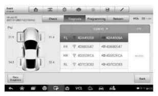
Figure 4-13 Sample No DTC Screen
