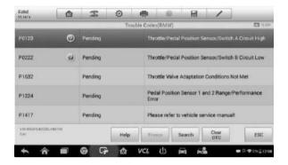
Figure 5-16 Sample DTC & FFD Screen
