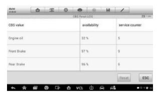
Figure 6-3 Sample Oil Reset Service Screen 2
